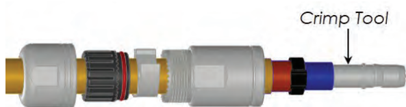
Step 5: Crimp terminal to conductor
