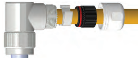
Step 4: Push cable into backshell. Slide components onto cable
