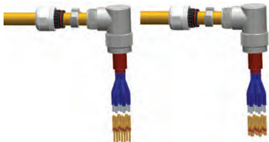
Step 7: Attach contacts to wire leads
