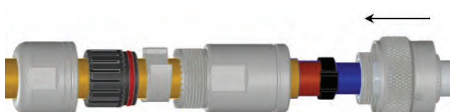
Step 6: Slide plug onto crimped terminal assembly
