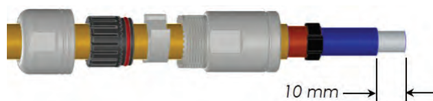
Step 6: Slide plug onto crimped terminal assembly
