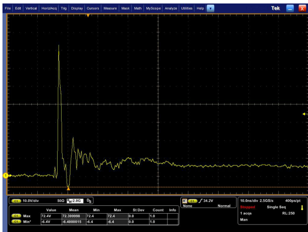
Figure 3. ESD Elamping Voltage Screenshot Positive 8 kV Eontact per IEE61000-4-2
