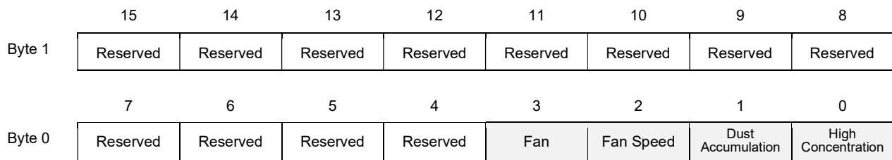
Figure 14. I 2 C Status Byte Details
