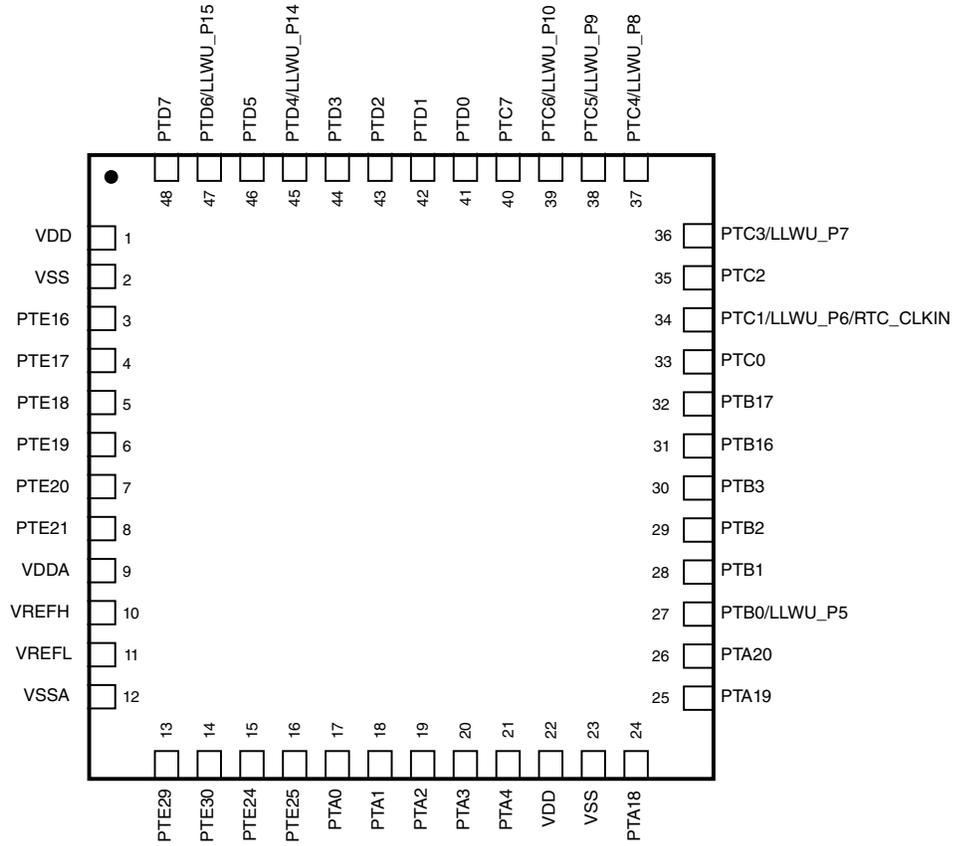
Figure 23. KL16 48-pin QFN pinout diagram
