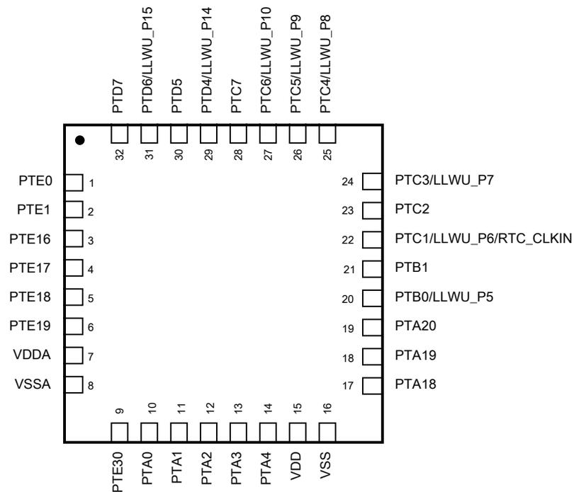
Figure 24. KL16 32-pin QFN pinout diagram
