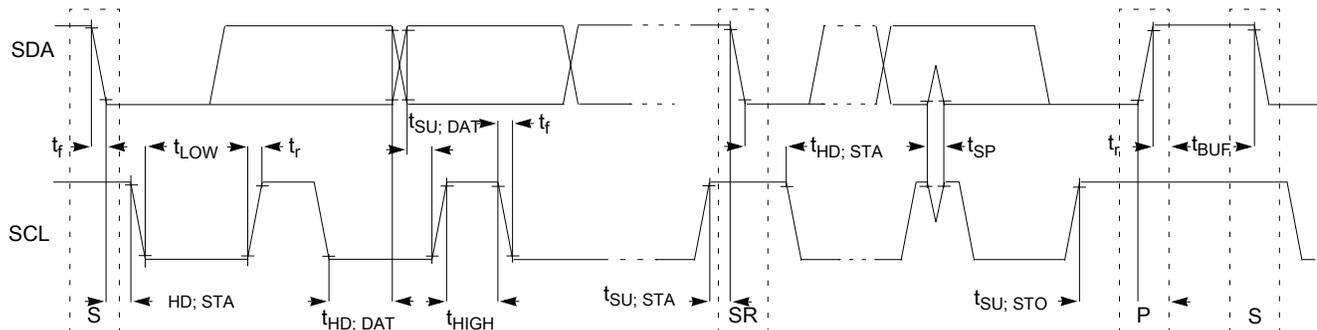
**Figure 17. Timing definition for devices on the I<sup>2</sup>C bus**
