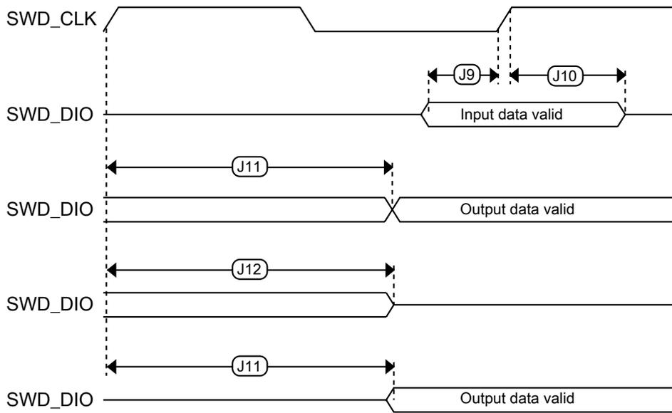
Figure 5. Serial wire data timing
