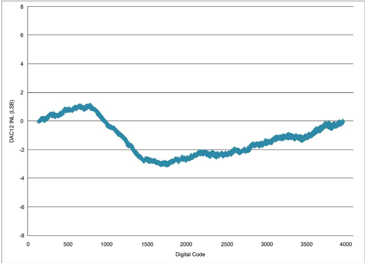
Figure 11. Typical INL error vs. digital code
