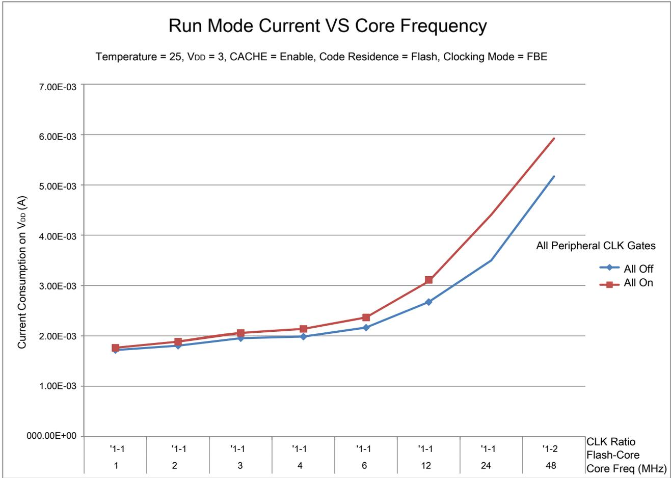
**Figure 2. Run mode supply current vs. core frequency**
