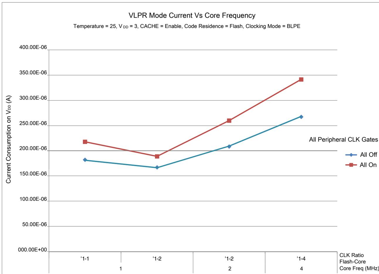
Figure 3. VLPR mode current vs. core frequency
