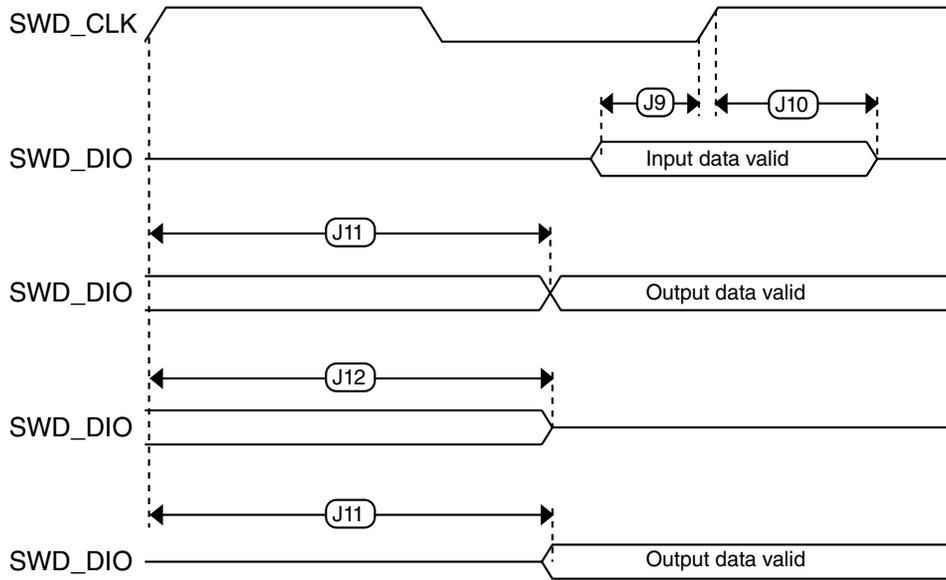
Figure 14. Serial wire data timing
