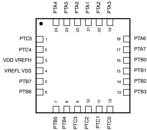
Figure 21. 24-pin QFN package
