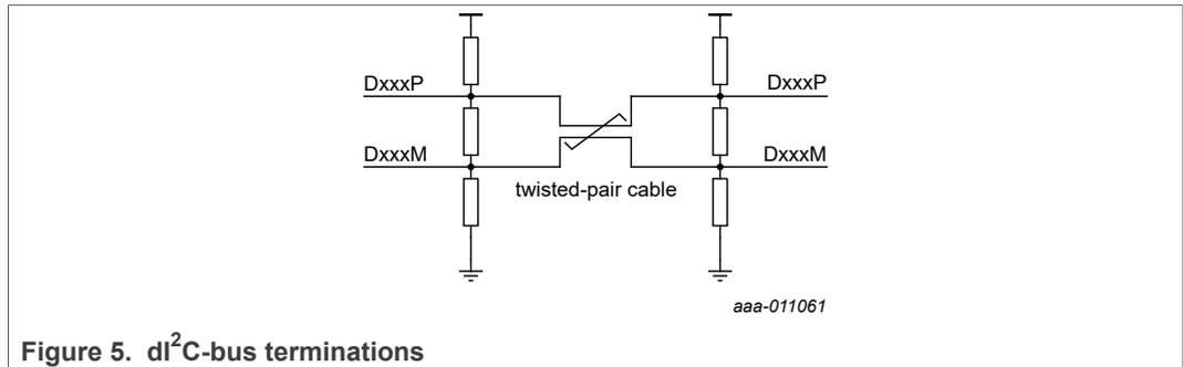
Figure 5. dl<sup>2</sup>C-bus terminations
