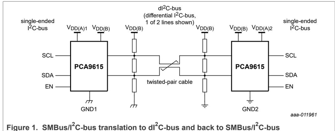
Figure 1. SMBus/I<sup>2</sup>C-bus translation to dI<sup>2</sup>C-bus and back to SMBus/I<sup>2</sup>C-bus
