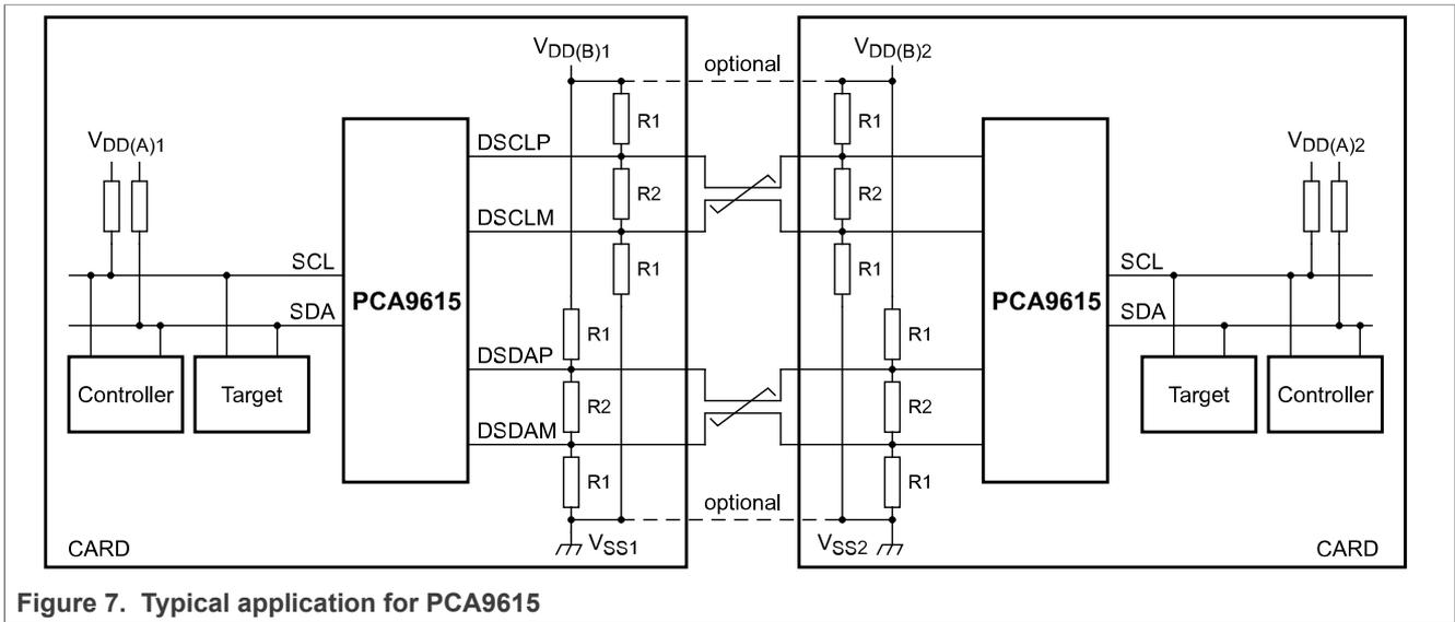
Figure 7. Typical application for PCA9615
