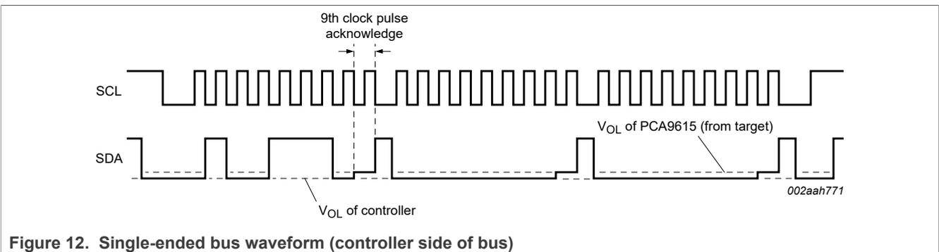
Figure 12. Single-ended bus waveform (controller side of bus)
