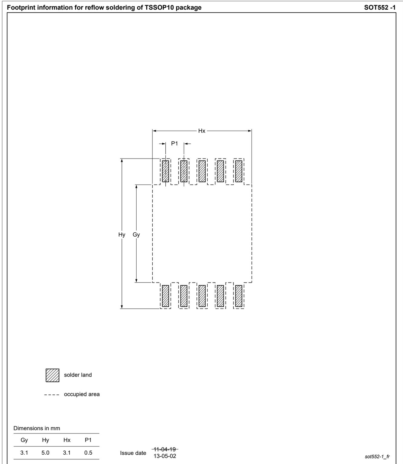
Figure 20. PCB footprint for SOT552-1 (TSSOP10); reflow soldering
