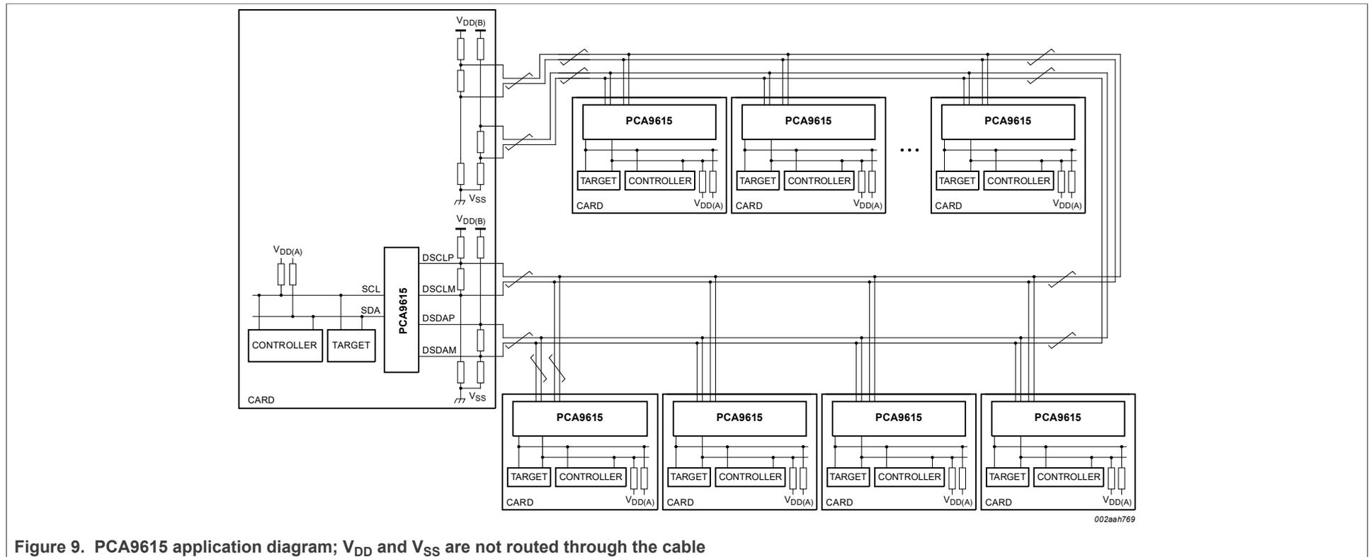
Figure 9. PCA9615 application diagram; V<sub>DD</sub> and V<sub>SS</sub> are not routed through the cable
