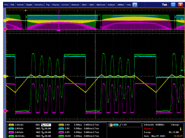
Figure 26. Valley Detection in DCM. Positive Line Cycle on Left, Negative on Right
