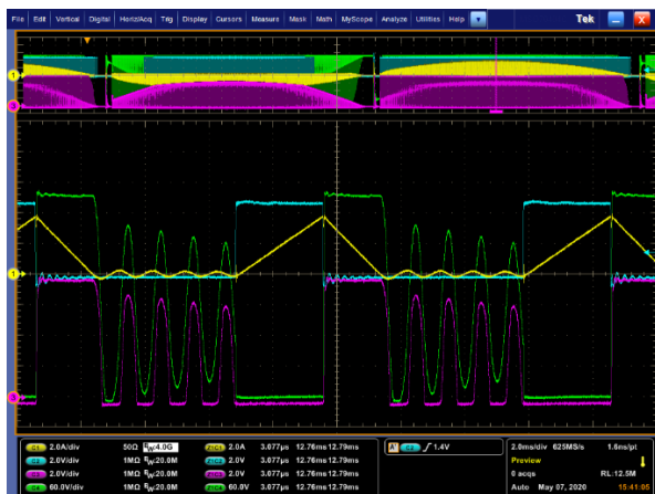
Figure 26. Valley Detection in DCM. Positive Line Cycle on Left, Negative on Right
