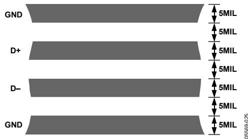
Figure 35. Typical Arrangement of Signal Tracks
