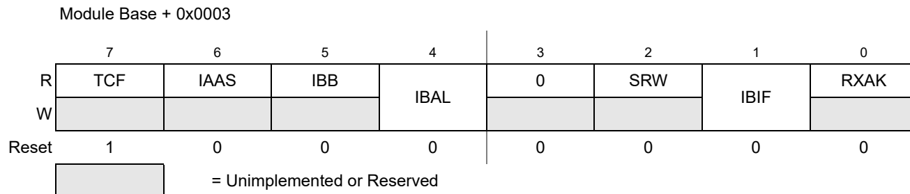
Figure 16-7. IIC Bus Status Register (IBSR)
