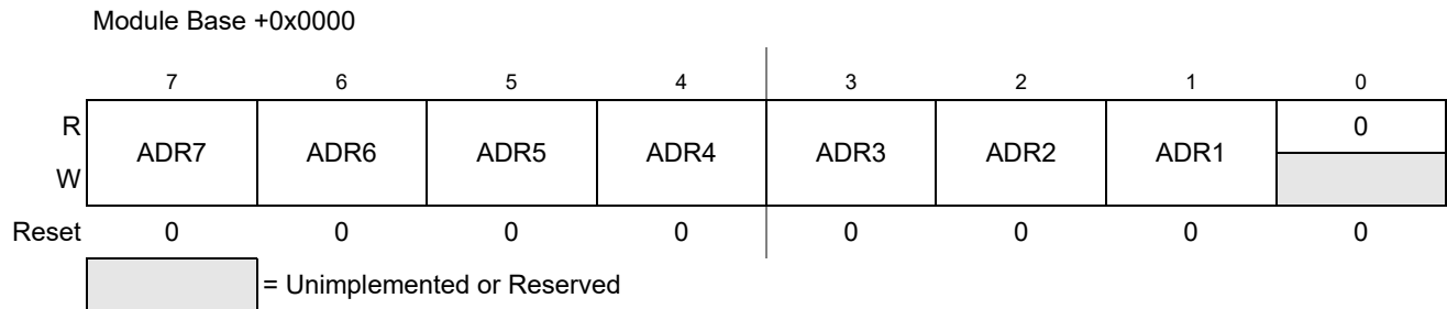
Figure 16-3. IIC Bus Address Register (IBAD)
