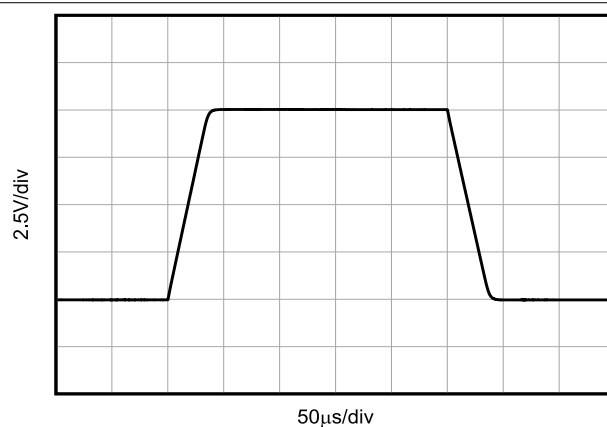
Figure 5-18. Large-signal Step Response ( G = 1 , R_L = 10\text{ k}\Omega , C_L = 200\text{ pF} )
