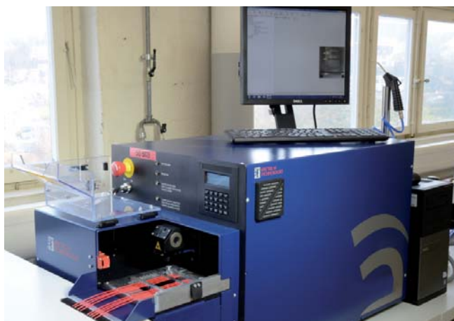
Automatic laser stripping
