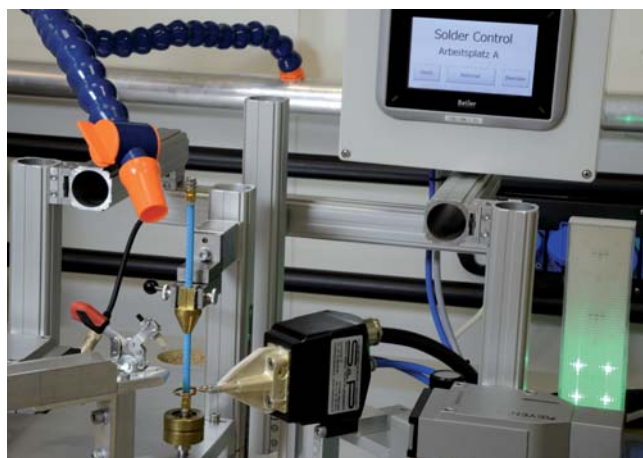
Temperature controlled soldering
