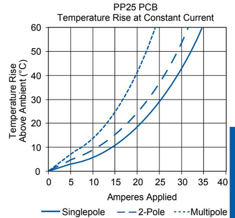
Current - Temperature Derating per IEC 60512-5-2 Test 5B
