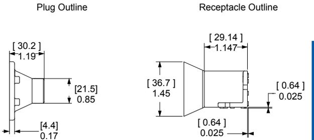
See our innovative MARC Connector that offers straight-on or rotational blindmate capability. MARC holds 6 PP15/45 power contacts and 2 PP15/45 premate ground contacts in a high temperature housing. Visit our website, [www.andersonpower.com](http://www.andersonpower.com) to learn more.
