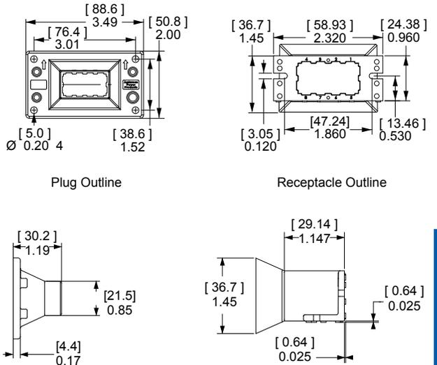
See our innovative MARC Connector that offers straight-on or rotational blindmate capability. MARC holds 6 PP15/45 power contacts and 2 PP15/45 premate ground contacts in a high temperature housing. Visit our website, [www.andersonpower.com](http://www.andersonpower.com) to learn more.
