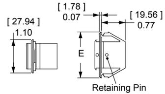
NOTE: Retaining pins are used to secure and position Powerpole® housings in one of two positions in receptacle shells.
