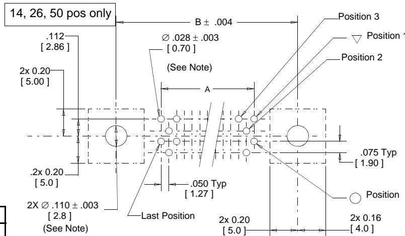
Note: Plated through holes for .062" board thickness.
