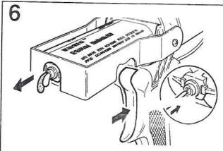
Squeeze trigger to expel a small amount of adhesive. Ensure that both components flow freely. Clear orifice of hardened material if necessary.
