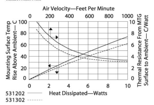
Thermal resistance value is based on a 75°C rise in natural convection
