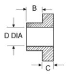
Note: A single gate extension, not to exceed 0.64mm (0.025") in length, is allowable on the outside of all shoulder washers.
