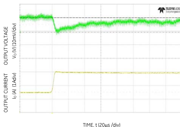
Figure 10. Transient Response to Dynamic Load Change from 50% to 100% at 12Vin, C_{out}=6 \times 47\mu\text{F} + 1 \times 330\mu\text{F} , C_{Tune}=5600\text{pF} , R_{Tune}=300\Omega
