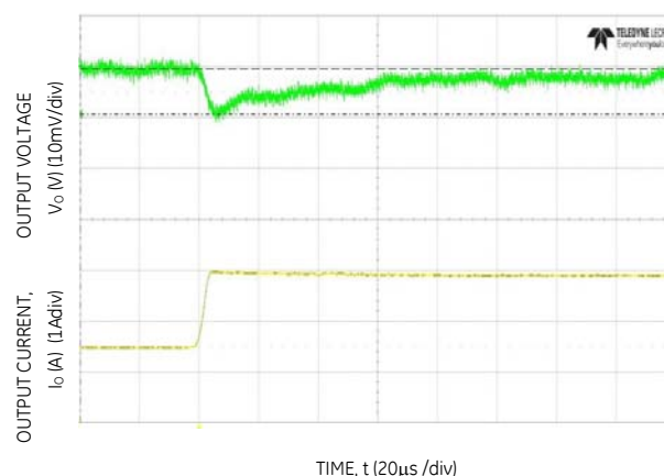
Figure 4. Transient Response to Dynamic Load Change from 50% to 100% at 12Vin, C_{out}=8 \times 47\mu\text{F} + 1 \times 330\mu\text{F} , C_{Tune}=5.6\text{nF} , R_{Tune}=300\Omega
