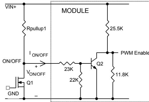
Figure 43. Circuit configuration for using negative On/Off logic.
