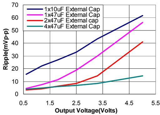
Figure 41. Output ripple voltage for various output voltages with external 1x10 μF, 1x47 μF, 2x47 μF or 4x47 μF ceramic capacitors at the output (12A load). Input voltage is 12V.
