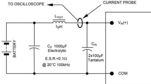
NOTE: Measure input reflected ripple current with a simulated source inductance ( $L_{TEST}$ ) of 1µH. Capacitor  $C_S$  offsets possible battery impedance. Measure current as shown above.
