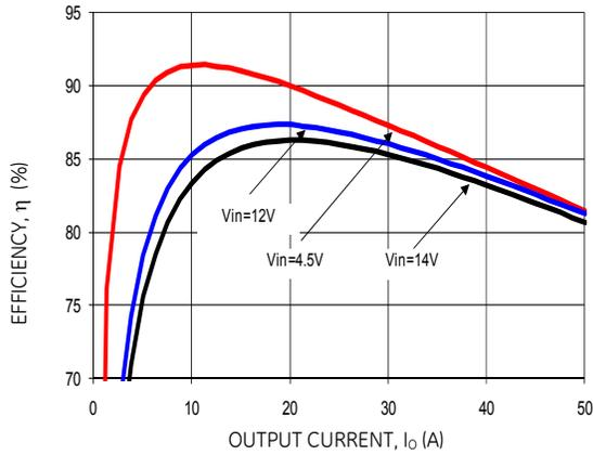
Figure 1. Converter Efficiency versus Output Current.
