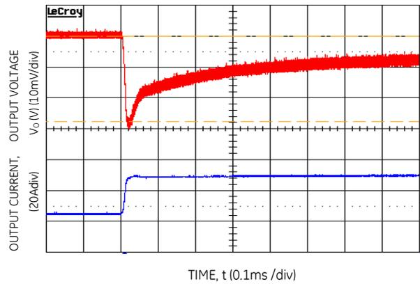
Figure 10. Transient Response to Dynamic Load Change from 50% to 100% at 12Vin,  $C_{ext} = 5 \times 47 \mu F + 13 \times 330 \mu F$  polymer,  $C_{Tune} = 120nF$ ,  $R_{Tune} = 180ohms$
