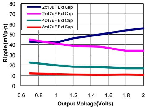
Figure 23. Output ripple voltage for various output voltages with external 2x10  $\mu$ F, 2x47  $\mu$ F, 4x47  $\mu$ F or 8x47  $\mu$ F ceramic capacitors at the output (50A load). Input voltage is 12V.
