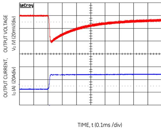
Figure 16. Transient Response to Dynamic Load Change from 50% to 100% at 12Vin,  $C_{ext} = 5 \times 47\mu F + 8 \times 330\mu F$  polymer,  $C_{Tune} = 47nF$ ,  $R_{Tune} = 220ohms$
