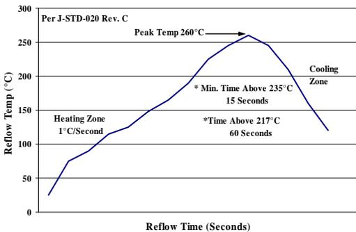
Figure 28. Recommended linear reflow profile using Sn/Ag/Cu solder.
