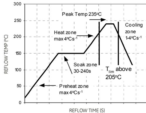
Figure 26. Reflow Profile for Tin/Lead (Sn/Pb) process.
