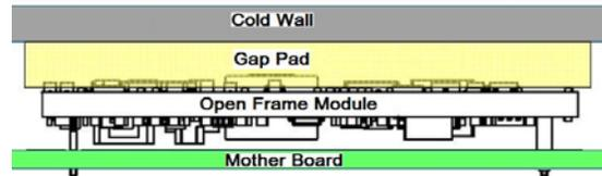
Figure 22. Cold Wall Mounting
