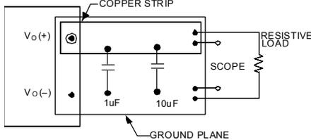
NOTE: All voltage measurements to be taken at the module terminals, as shown above. If sockets are used then Kelvin connections are required at the module terminals to avoid measurement errors due to socket contact resistance.
