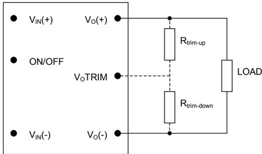
**Figure 12. Circuit Configuration to Trim Output Voltage.**
