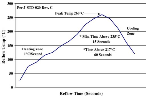
Figure 27. Recommended linear reflow profile using Sn/Ag/Cu solder.
