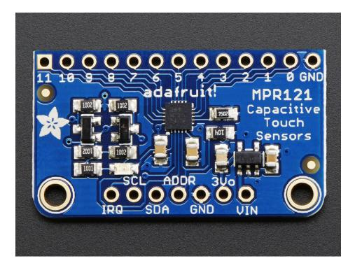
The little chip in the middle of the PCB is the actual MPR121 sensor that does all the capacitive sensing and filtering. We add all the extra components you need to get started, and 'break out' all the other pins you may want to connect to onto the PCB. For more details you can check out the schematics in the Downloads page.
