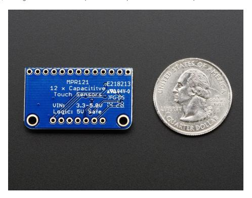
The MPR121 has support for only I2C, which can be implemented with nearly any microcontroller. You can select one of 4 addresses with the ADDR pin, for a total of 48 capacitive touch pads on one I2C 2-wire bus. Using this chip is a lot easier than doing the capacitive sensing with analog inputs: it handles all the filtering for you and can be configured for
