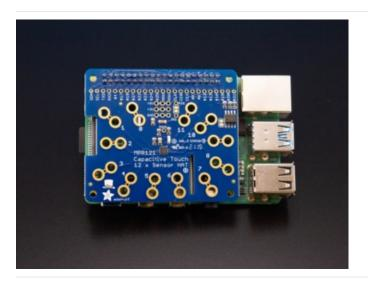
Simply solder (https://adafru.it/drl) the header provided with the HAT onto the HAT, and attach the HAT to the Pi.
