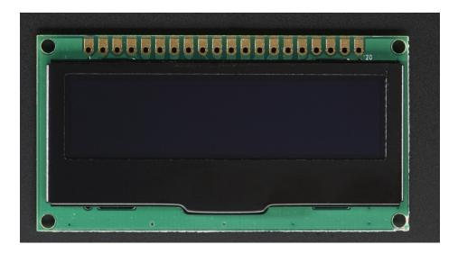
The pins on these modules are not well marked, but the one on left is #1 and the pins increment in order until the one on the very right, #20
