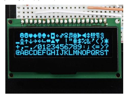
The driver chip, SSD1305 can communicate in three ways: 8-bit, I2C or SPI. Personally we think SPI is the way to go, only 4 or 5 wires are required and its very fast. The OLED itself requires a 3.3V power supply and 3.3V logic levels for communication. We include a breadboard-friendly level shifter that can convert 3V or 5V down to 3V, so it can be used with 5V-logic devices like Arduino.
