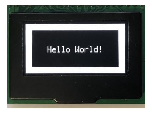
If you have the 2.3" 128x32 OLED Display, here's what the final output looks like with the height set to 32 and the border size set to 5:
