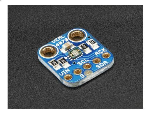
This little sensor is a great way to add UV light sensing to any microcontroller project. The VEML6070 from Vishay has a true UV A light sensor and an I2C-controlled ADC that will take readings and integrate them for you over  $^{\circ}$ 60ms to 500ms.
