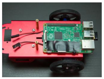
If you aren't using Pi HAT standoffs to hold the motor HAT place a piece of electrical tape across the HDMl connector side of the Pi. This will help prevent the motor HAT from getting pushed down into the connectors and shorting out. If you are using the standoffs you can place them over the front mounting holes of the Pi (not shown).
