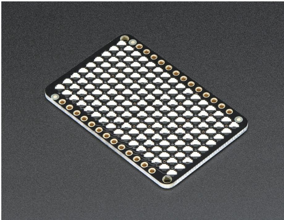
The IS31FL3731 is a nice little chip - it can use 2.7-5.5V power and logic so its flexible for use with any microcontroller.
