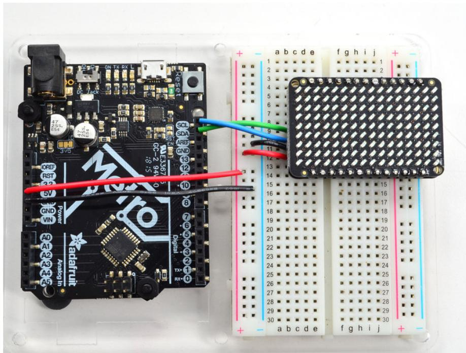
You can easily wire this breakout to any microcontroller, we'll be using an Arduino. For another kind of microcontroller, as long as you have I2C pins available, just check out the library, then port the code.
