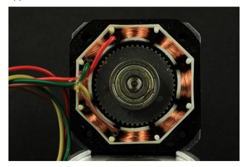
Stepper motors are DC motors that move in discrete steps. They have multiple coils that are organized in groups called "phases". By energizing each phase in sequence, the motor will rotate, one step at a time.
