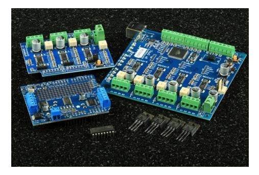
Driving a stepper motor is a bit more complicated than driving a regular brushed DC motor. Stepper motors require a stepper controller to energize the phases in a timely sequence to make the motor turn.
