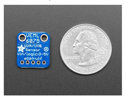
This UV sensor works great with 3 or 5V power or logic, its nice and compact, and its easy to use with any I2C-capable microcontroller. We have example code and libraries for Arduino (https://adafru.it/CCj) and CircuitPython/Python (https://adafru.it/CCk).
