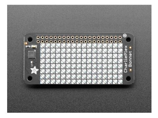
The IS31FL3731 is a nice little chip - and it runs happily over 3.3V power. Inside is enough RAM for 8 separate frames of display memory so you can set up multiple frames of an animation and flip them to be displayed with a single command. Since it uses I2C, it takes up only the SDA/SCL pins on your Pi and can share those pins with other I2C devices and sensors.
