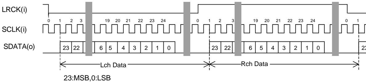
Figure 3. Serial Data Timing (I<sup>2</sup>S Slave mode, FSYNC: Don't care.)
