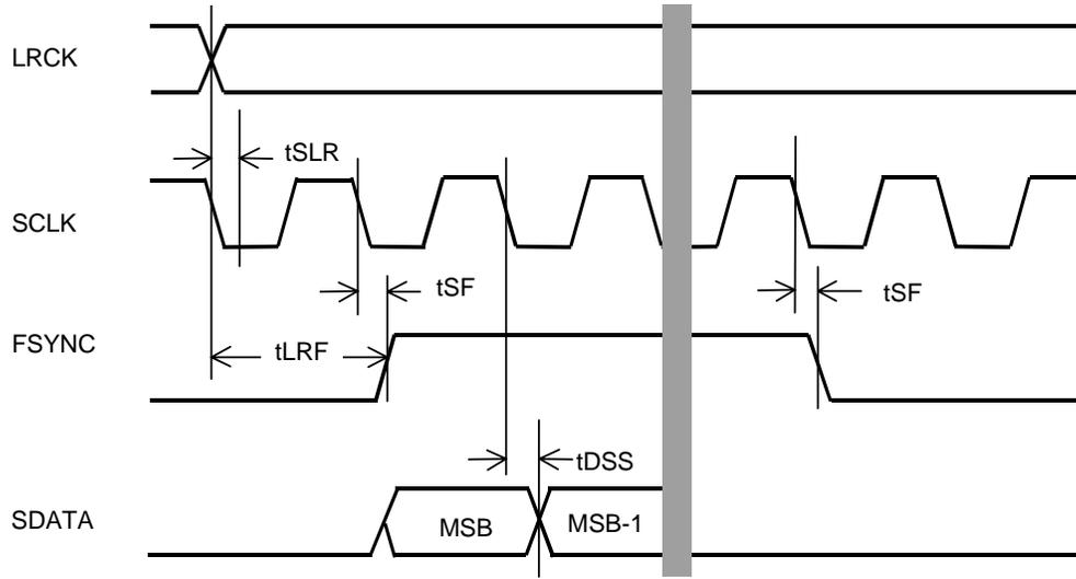
Serial Data Timing (Master Mode & I<sup>2</sup>S Master Mode, DFS = "L")
