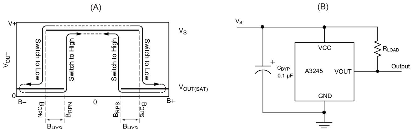
Figure 1: Switching Behavior of Omnipolar Switches. In Panel A, on the horizontal axis, the B+ direction indicates increasing south polarity magnetic field strength, and the B- direction indicates decreasing south polarity field strength (including the case of increasing north polarity). This behavior can be exhibited when using a circuit such as that shown in panel B.
