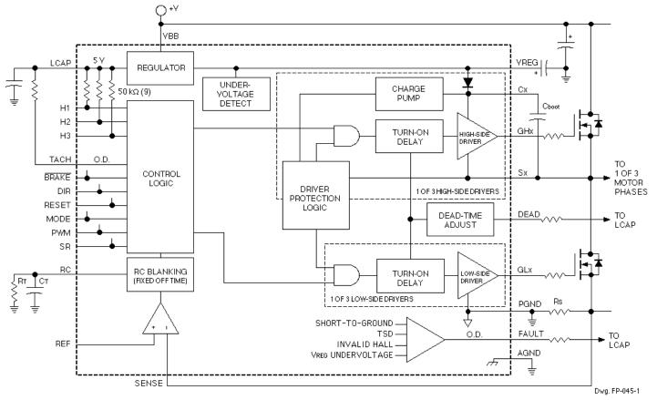
PWM input can be used to provide speed/torque control, allowing the internal current control circuit to set the maximum current limit.
