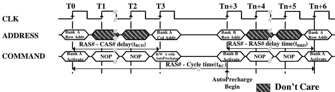
**Figure 3. BankActivate Command Cycle (Burst Length = n)**
