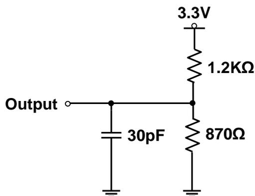
**Figure 18.1 LVTTL D.C. Test Load (A)**
