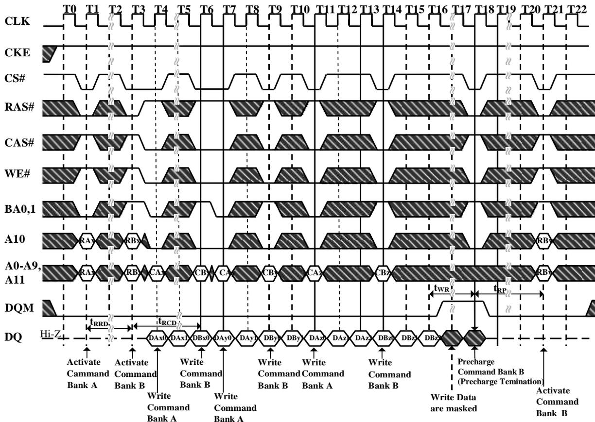
Figure 42. Precharge Termination of a Burst
