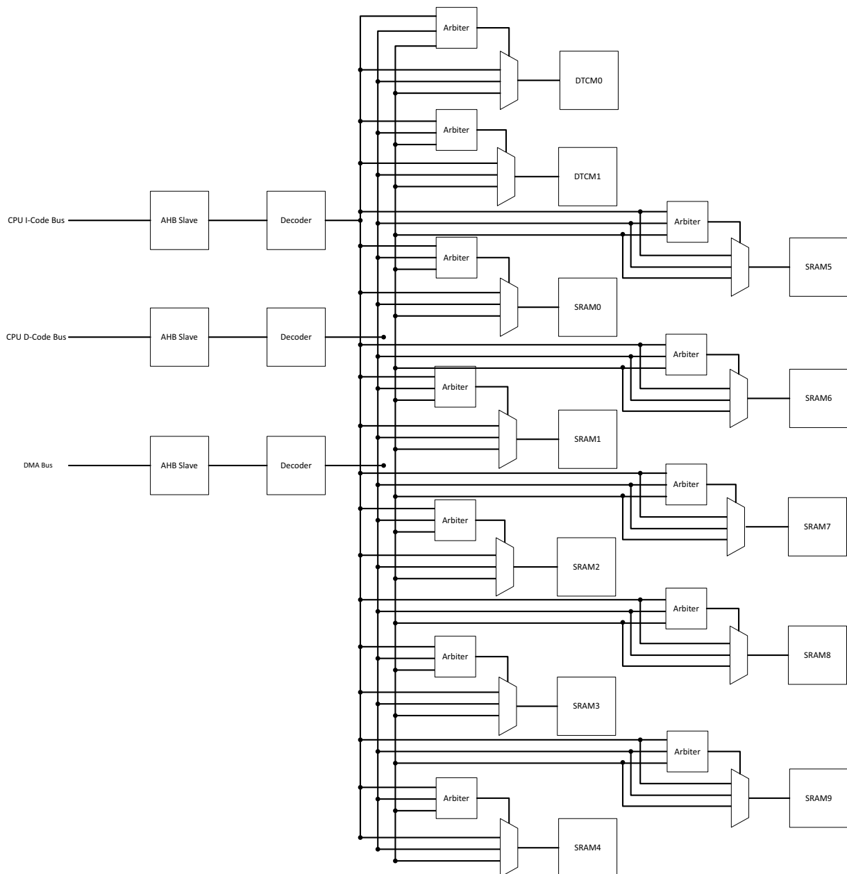
Figure 8. Block diagram for the SRAM Interface
