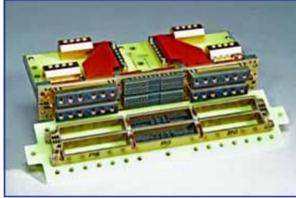
Line Replaceable Module (LRM) board level interconnects enhanced with RADSOK® contacts.
