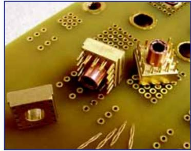
The RADSOK® PowerBlok™ provides a high current single-point connection to the PCB with the proven reliability of compliant pin signals. The PowerBlok™ is designed to bring up to 70 Amperes to the board, utilizing our custom 3.0mm RADSOK® design. The compliant pins are press-fit into the board to secure a solid connection and even flow.
