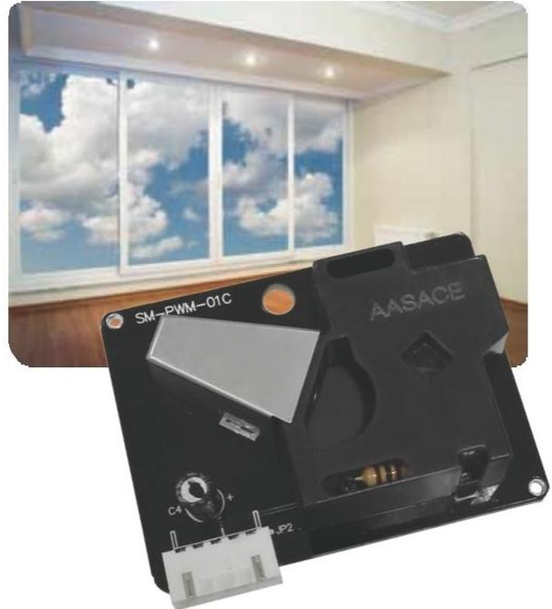
SM-PWM-01C is a dust sensor that detects the dust particle concentration in air by using optical sensing method. An infrared light emitting diode (IR LED) and a photo-sensor are optically arranged in the device. The photo-sensor detects the reflected IR LED light by dust particles in air.
