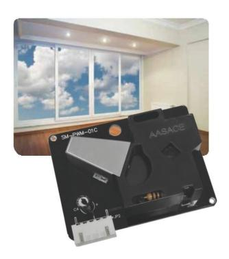
SM-PWM-01C is a dust sensor that detects the dust particle concentration in air by using optical sensing method. An infrared light emitting diode (IR LED) and a photo-sensor are optically arranged in the device. The photo-sensor detects the reflected IR LED light by dust particles in air.
