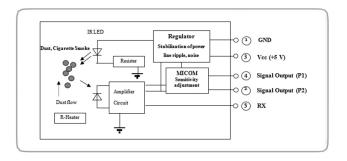
P1: small particle (1~2  $\mu$ m), P2: large particle (3 ~10  $\mu$ m)
