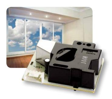
SM-PWM-01A is a dust sensor that detects the dust particle concentration in air by using optical sensing method. An infrared light emitting diode (IR LED) and a photo-sensor are optically arranged in the device. The photo-sensor detects the reflected IR LED light by dust particles in air.
