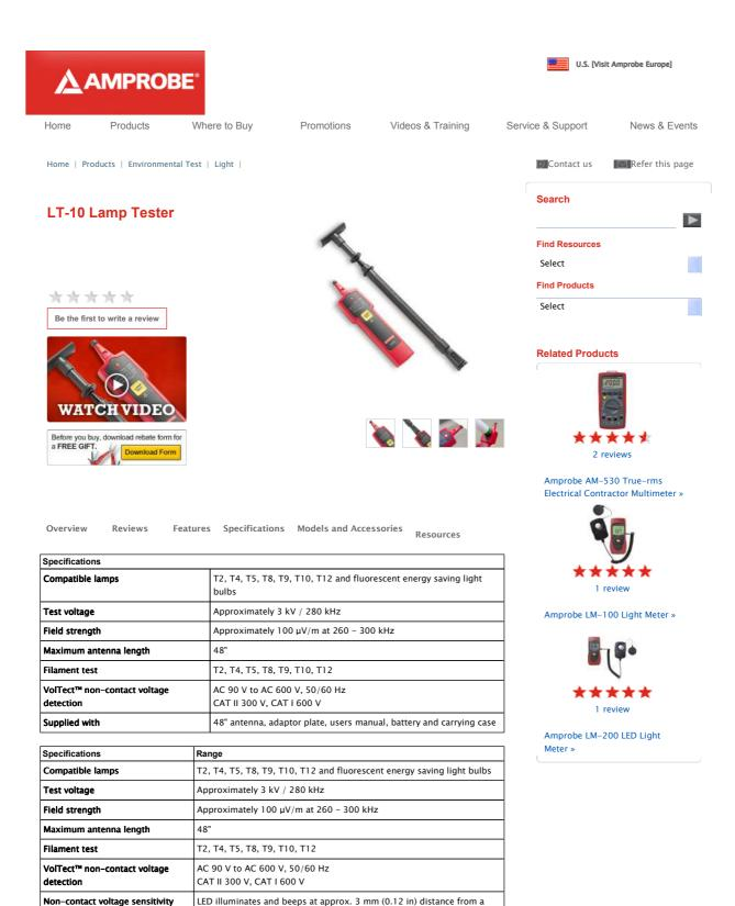
LED illuminates and beeps at approx. 5 mm (0.2 in) distance from a wire
