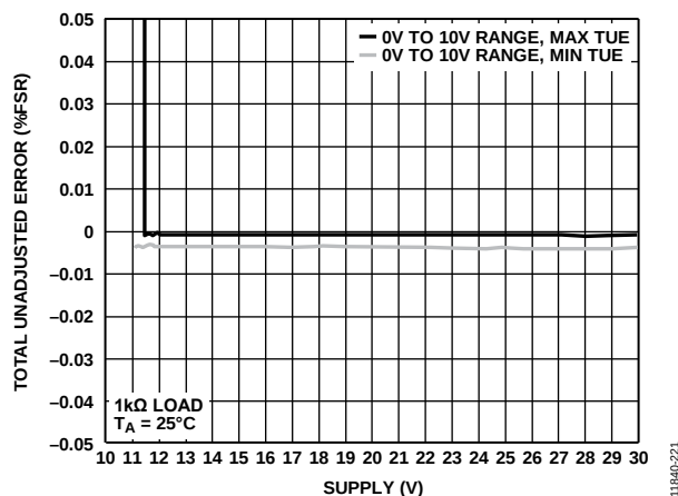
Figure 20. Total Unadjusted Error vs. AV_{DD1}/AV_{SS} Supply
