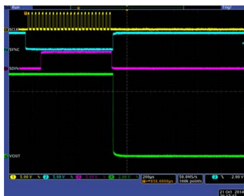
Figure 61. Software Full Reset Glitch from Full Scale with Output Loaded, \pm 10 V Range
