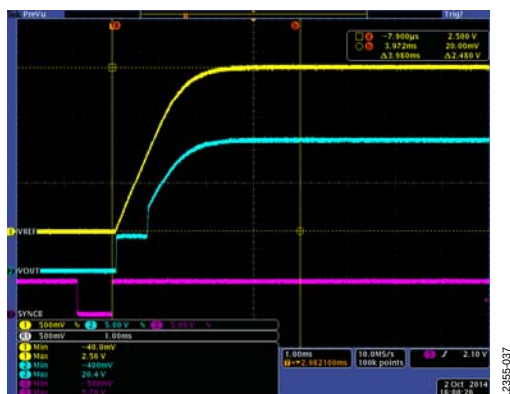
Figure 36. Reference Output Voltage Turn On Transient
