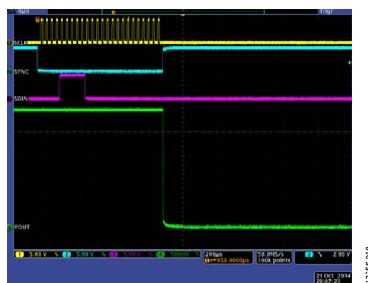
Figure 58. Software Full Reset Glitch from Full Scale with Output Loaded, 0 V to 5 V Range
