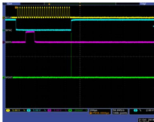
Figure 60. Software Full Reset Glitch from Zero Scale with Output Loaded, 0 V to 5 V Range
