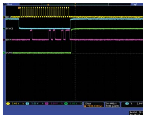
Figure 64. Output Range Change Glitch, 0 V to 5 V Range
