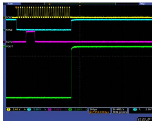
Figure 63. Software Full Reset Glitch from Zero Scale with Output Loaded, \pm 10 V Range
