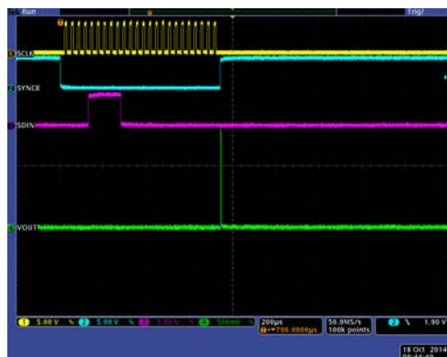
Figure 62. Software Full Reset Glitch from Midscale with Output Loaded, \pm 10 V Range
