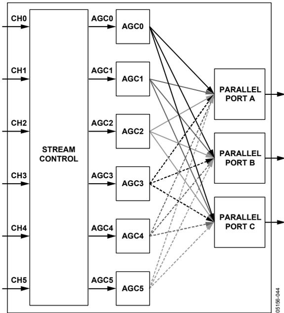
Figure 55. Block Diagram of the Output Data Router
