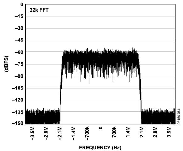
Figure 30. WCDMA Carrier AIN = 151.5 MHz; Encode = 92.16 MSPS
