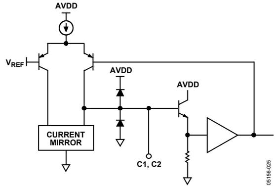
Figure 35. ADC Compensation Pins, C1 and C2
