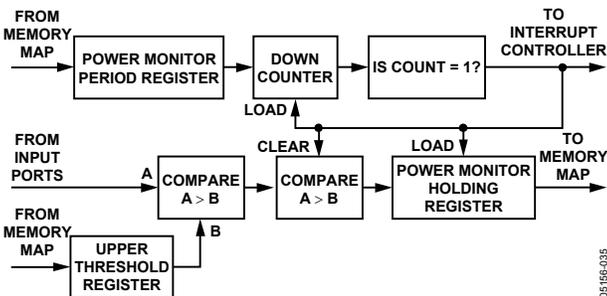
Figure 46. ADC Input Threshold Crossing Block Diagram
