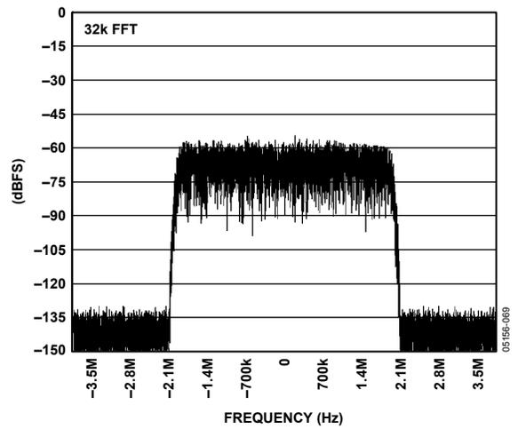
Figure 29. WCDMA Carrier AIN = 70 MHz; Encode = 92.16 MSPS
