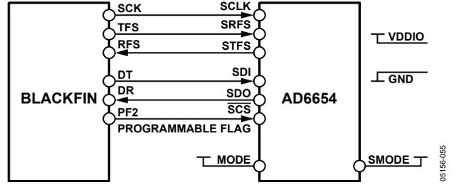
Figure 74. SPORT Mode Serial Port Connections to Blackfin
