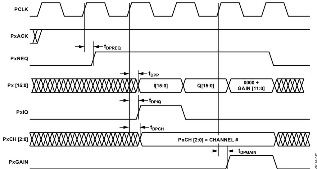
Figure 58. Interleaved I/Q Mode with an AGC Gain Word
