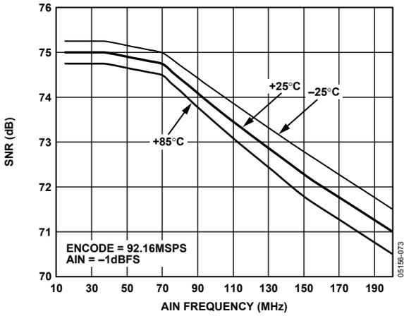
Figure 19. ADC Noise vs. Analog Frequency (46.08 MHz BW)
