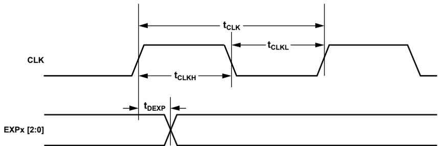
Figure 7. Gain Control Word Output Switching Characteristics
