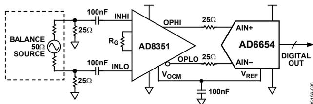
Figure 40. ADC Driving Application Using Differential Input
