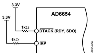
Figure 75.  $\overline{\text{DTACK}}$ ,  $\overline{\text{SDO}}$ ,  $\overline{\text{IRP}}$  Pull-Up Resistor Circuit
