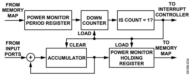
Figure 45. ADC Input Mean Power Monitoring Block Diagram
