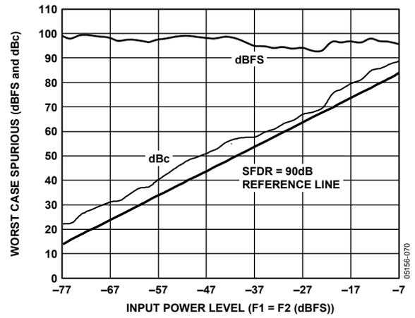
Figure 32. Two Tone SFDR at 55 MHz and 56 MHz
