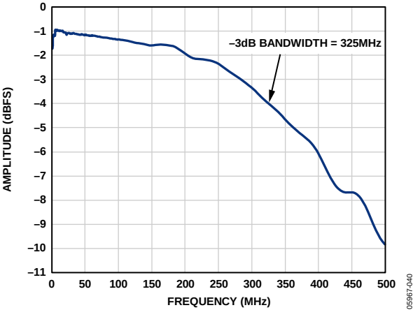
Figure 53. Full-Power Bandwidth vs. Frequency, AD9222-50
