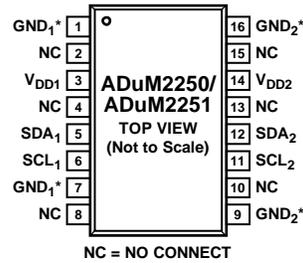
\*PIN 1 AND PIN 7 ARE INTERNALLY CONNECTED. CONNECTING BOTH TO GND<sub>1</sub> IS RECOMMENDED. PIN 9 AND PIN 16 ARE INTERNALLY CONNECTED. CONNECTING BOTH TO GND<sub>2</sub> IS RECOMMENDED.
