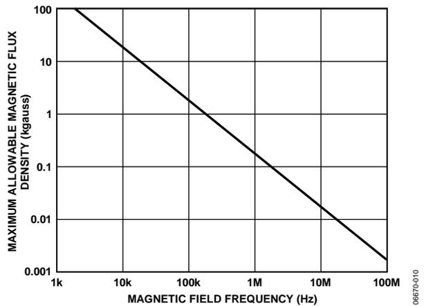
Figure 10. Maximum Allowable External Magnetic Flux Density
