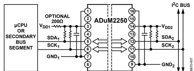
Figure 7. Typical Isolated I<sup>2</sup>C Interface Using ADuM2250
