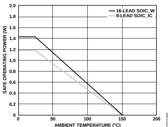
Figure 3. Thermal Derating Curve, Dependence of Safety Limiting Values with Case Temperature per DIN V VDE V 0884-10
