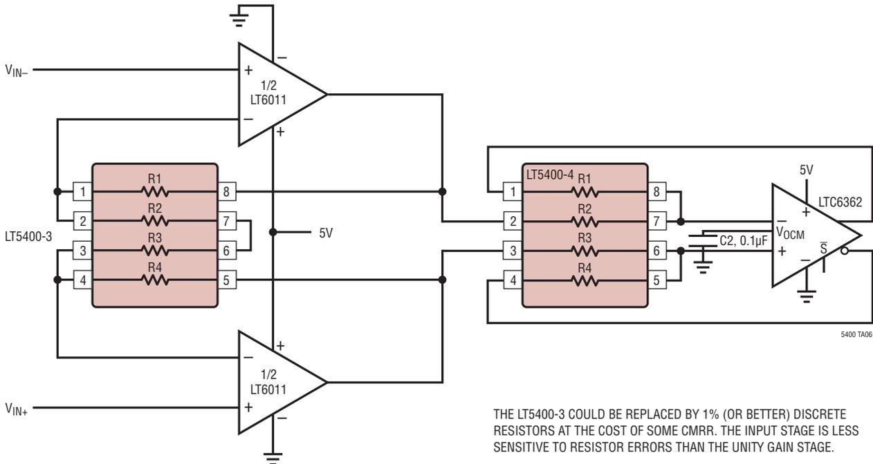
THE LT5400-3 COULD BE REPLACED BY 1% (OR BETTER) DISCRETE RESISTORS AT THE COST OF SOME CMRR. THE INPUT STAGE IS LESS SENSITIVE TO RESISTOR ERRORS THAN THE UNITY GAIN STAGE.
