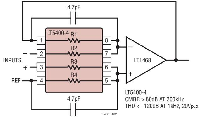
Low Noise Reference Divider with Op Amp Input Bias Current Balancing
