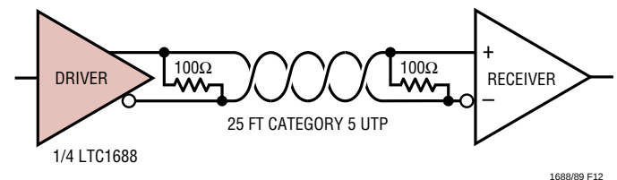
Figure 12. 100Mbps Differential Data Connection
