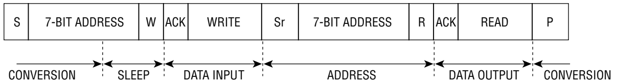
Figure 6. Write, Read, Start Conversion
